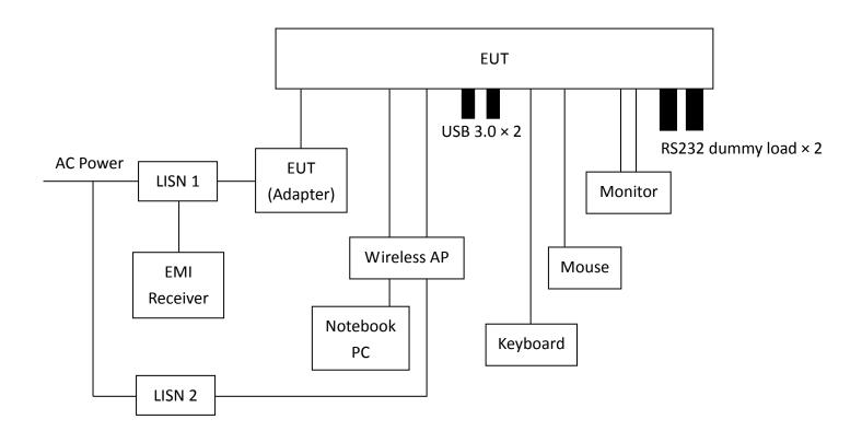
The EUT along with its peripherals were placed on a 1.0 meter(W)×1.5meter(L) and 0.8 meter in height wooden table and the EUT was adjusted to maintain a 0.4meter space from a vertical reference plane. The EUT was connected to power mains through a Artificial Mains Network (LISN), which provided 50 ohm coupling impedance for measuring instrument and the chassis ground was bounded to the horizontal ground plane of shielded room.
